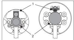
When pushed in, the mounting pin (2) locks automatically. To undo the mounting pin (2), push the tab washer (1) upwards and pull out the mounting pin (2).
